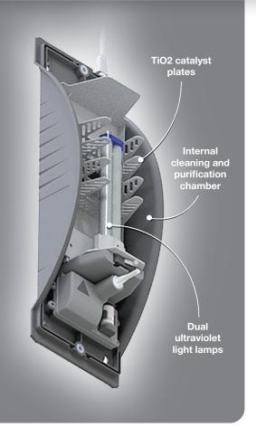
The dual ultraviolet lamps within the various units, operate at the peak UVC wavelengths in the presence of TiO2 catalyst plates, enclosed within our reflective internal cleaning and purification chamber. This creates Germicidal Irradiation, PCO – Photocatalytic Oxidation, Hydroxyl Radicals and Superoxide Ions and optional Ozone, which leave the unit as Plasma Quatro.
